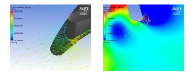
Fig. 8 CFD calculation of inlet recirculation
