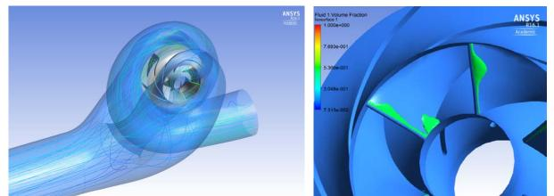
Fig. 7 CFD calculation of bubble formation
