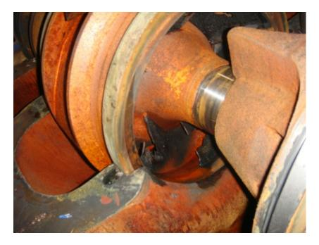
Fig.4 Cavitation damage due to the recirculation
