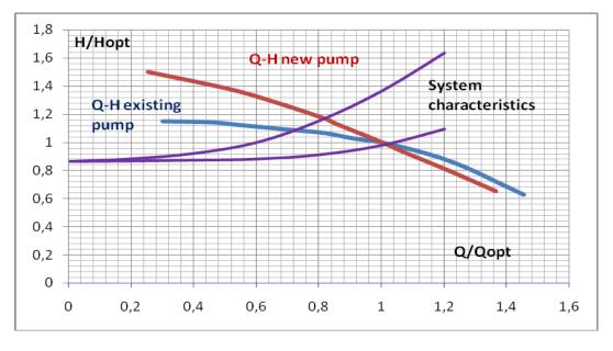
Fig.5 Dimensionless Q-H Characteristic of the new pump compare with existing one
