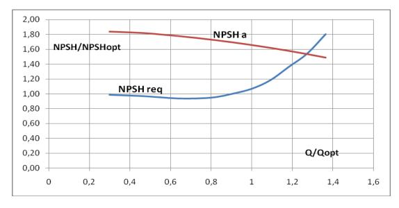
Fig.3 Dimensionless characteristic of NPSH req and NPSH a
