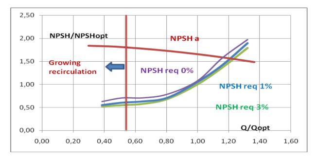
Fig.6 Dimensionless Q-NPSH Characteristic of the new pump
